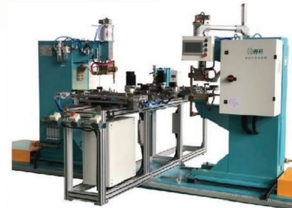
Automatic spot weld machine for battery shell plate
