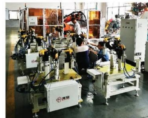
Automotive Battery Bracket Spot Welding Workstation
