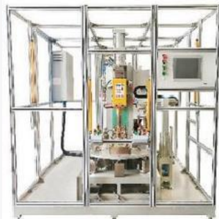
Six-Station Automatic Spot Welding Machine for Automotive Shock Absorber Bracket
