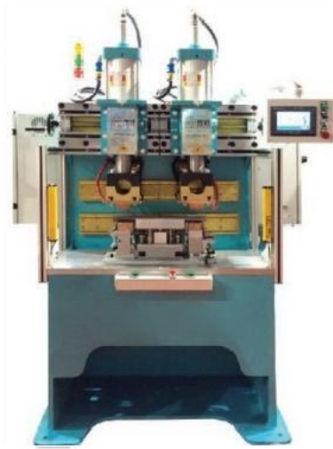
Seat Angle adjuster double head convex welding machine
