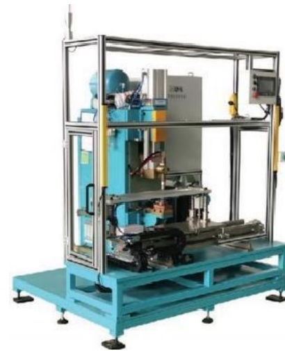
Motor pole shoe automatic projection welding machine
