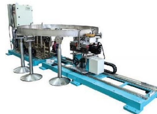
Special machine for roll welding of corrugated pipes
