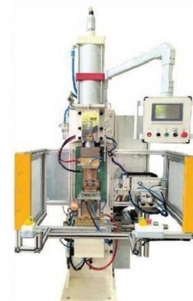
Automotive latch hot riveting machine
